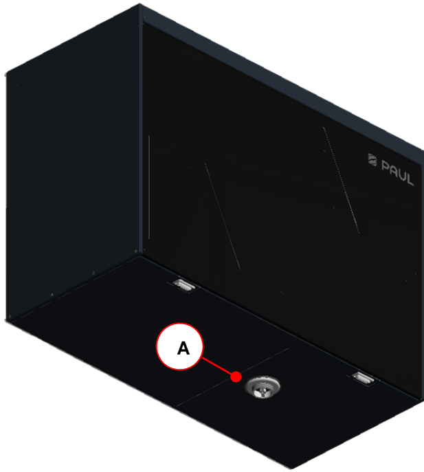
Fig 29: Connector of the condensate drain version LEFT
